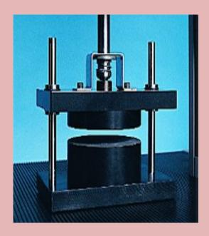
Circular compression jig with linear bearing guides to maintain parallel alignment of face plates. Compression testing of corrugated cardboard and paper products. A test piece of corrugated cardboard or paper is placed between the platens of a crush tester with the flutes perpendicular to the platens. It is then subjected to compression until failure. The maximum force sustained by the test piece is measured.
