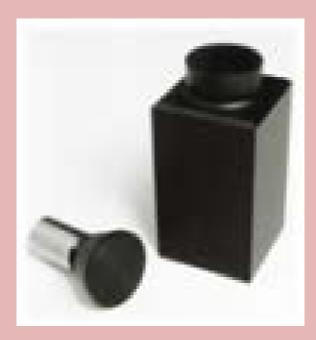
Circular direct compression platens for performing General purpose low force compression tests.
