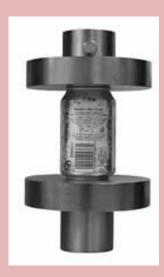
Round Compression Platens for large samples up to 200mm (7.9 in) in diameter.
