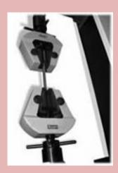
Capstan Action Parallel Wedge Grip supplied with straight cut faces for flat samples as standard. Capstan action enables the sample to be held tightly in the jaws before commencing the test. Tensile testing of flat or round rigid materials, general metallurgical and composite applications are stretching a sample to break and recording the relationship between force and extension.
