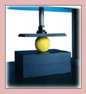
Rectangular direct compression platens for samples up to 175mm x 115mm (6.9 x 4.5 in) General compression testing for a wide range of materials and products for the purpose of determining one or more of the following compressive properties:
