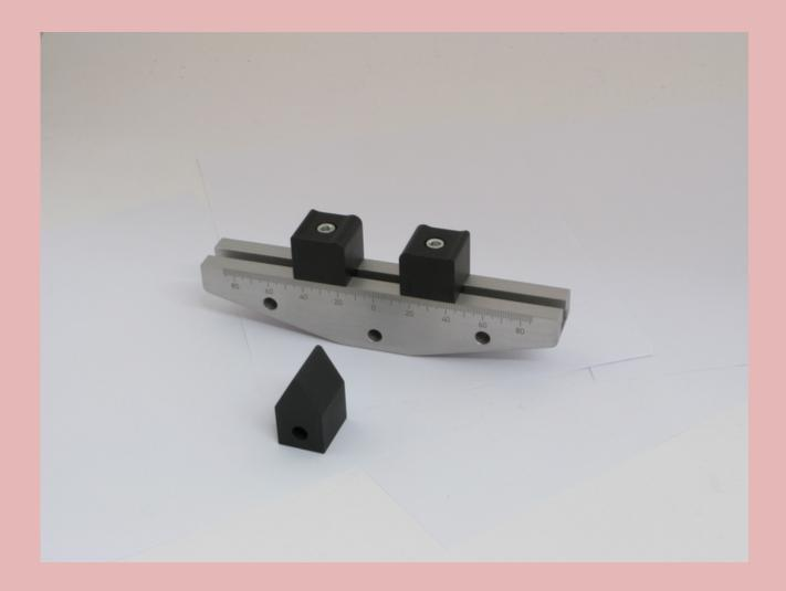
Three point bending fixture for large samples up to 600mm (24 in) in length. Mandrels different size as per requirement upto maximum capacity
