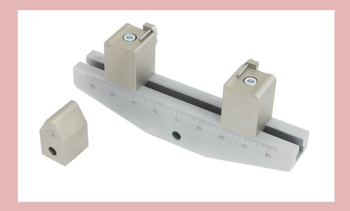
Three point bending fixture for large samples up to 600mm (24 in) in length. Mandrels different size as per requirement upto maximum capacity
