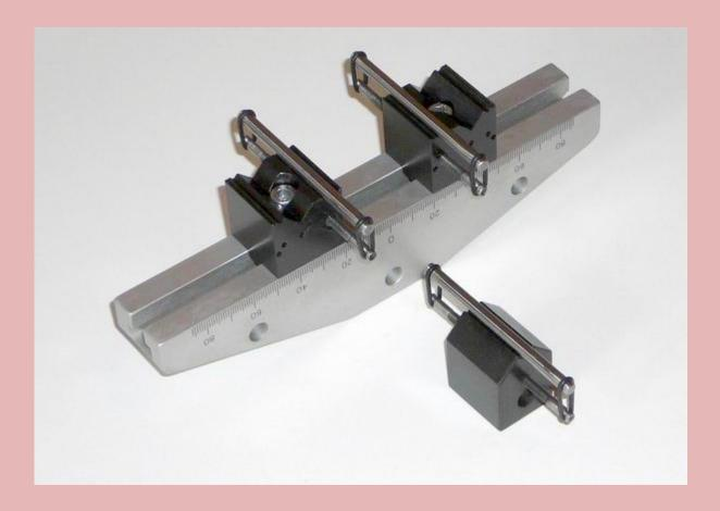
Three point bending fixture for large samples up to 600mm (24 in) in length. Mandrels different size as per requirement upto maximum capacity
