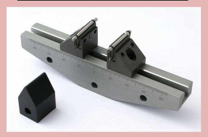
Three point bending fixture for large samples up to 600mm (24 in) in length. Mandrels different size as per requirement upto maximum capacity
