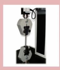
General purpose sliding wedge, self tightening grips supplied with straight cut faces as standard. Two additional face options are available. Tensile testing of flat or round plastics and light metals etc. by stretching a sample to break and recording the relationship between force and extension.
